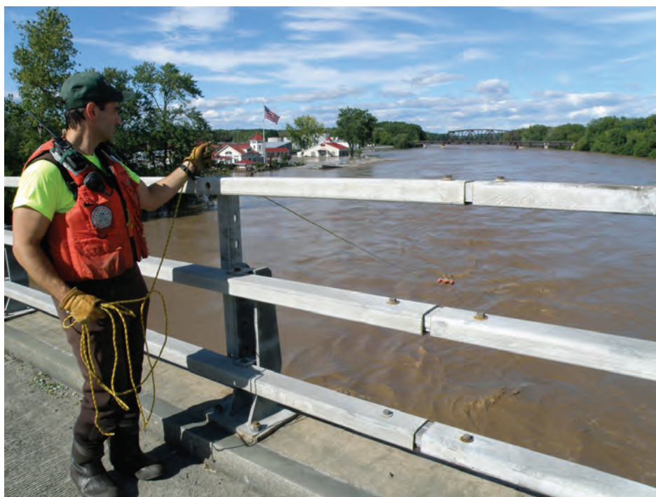
Figure 3. U.S. Geological Survey (USGS) hydrographer making a streamflow measurement using an acoustic Doppler current profiler (ADCP) at the Mohawk River at Freeman's Bridge at Schenectady, N.Y. (01354500) USGS streamgage. Photograph by Alicia Gearwar, USGS.
