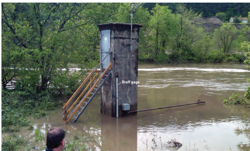
Figure 2. U.S. Geological Survey (USGS) hydrographer determining the outside stage at the Passumpsic River at Passumpsic, Vt. (01135500) USGS streamgage, May 27, 2011. Photograph by Richard Kiah, USGS.
